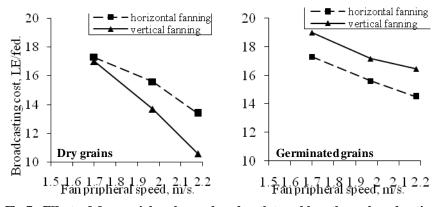
Fig.7: Effect of fan peripheral speed and outlet pathlength on broadcasting cost under 200 mm outlet path length with dry and germinated grains
