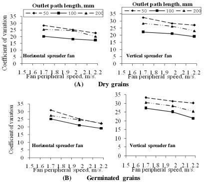
Fig.5: Effect of fan peripheral speed and outlet path on coefficient of variation for: (A) dry grains and (B) germinated grains
