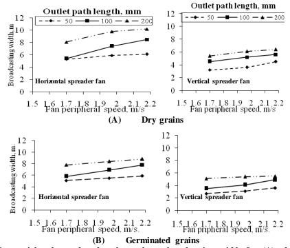
Fig.4: Effect of fan peripheral speed and outlet path on broadcasting width for (A): dry grains and (B) germinated grains
