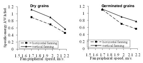
Fig.6: Effect of fan peripheral speed and outlet path length on specific energy under 100 mm outlet path length with dry and germinated grains
