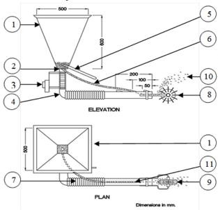
Fig. 2: A schematic diagram of the developed portable unit
